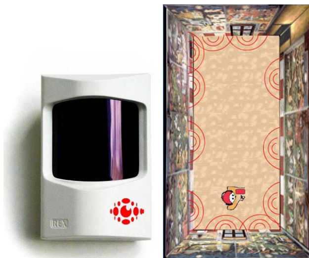
Figure 1. Infrared beacon and overview on an exemplary infrared installation in a single room (red semicircles indicate beacon positions and ranges).
